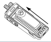
**2** To remove the battery, turn the radio off. Move the battery latch (A) into unlock position and hold, and slide the battery down and off the rails.
