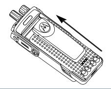
2 To remove the battery, turn the radio off. Move the battery latch (<sup>(A)</sup>) into unlock position and hold, and slide the battery down and off the rails.
