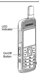
**NOTE:** Brightness is set via the manual brightness mode or auto brightness is controlled by the radio's photo sensor. The Home screen does not light up during a power up if the LED indicator is disabled (see *Turning the LED Indicator On or Off* on page 88).
